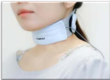
**C-STRETCH(TM) Swallowing count measurement tool
